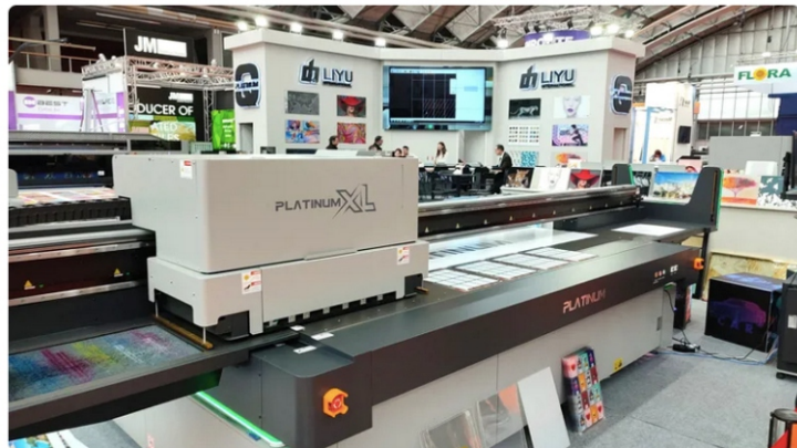
Liyu's new flagship flatbed, the KCXL+ can be fitted with 24 or 32 Ricoh Gen6 printheads
