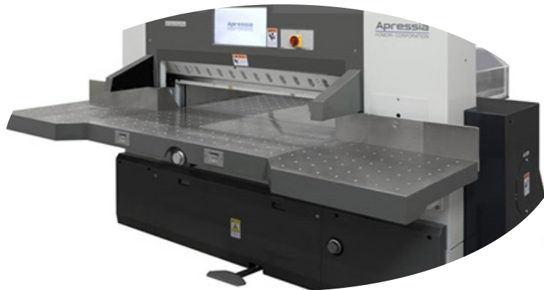
Apressia CT 137 - automated and programmable Hydraulic Clamp Cutter
