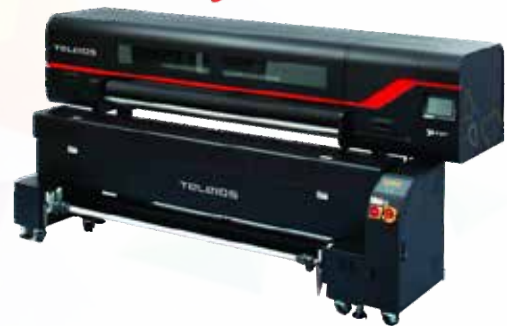
Roll to Roll Direct to Textile printing on cotton material (Fashion & Home Textile)
