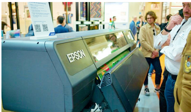
•Epson's SureColor R5000 is a 1.6m wide roll-to-roll device that uses resin ink. Credit: Nessan Cleary.
