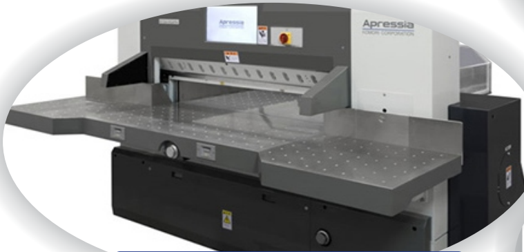
Apressia CT 137 - automated and programmable Hydraulic Clamp Cutter
