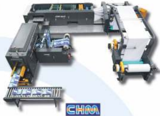
CHM COMPACT A4 CUT SIZE SHEETING AND PACKAGING PRODUCTION LINE CUTTING-SIZE SHEETING, SINGLE FEED PACKING
